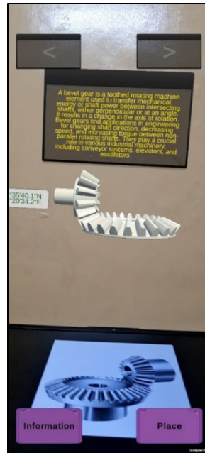
Figure 8. Bevel gear model with infographics and coordinates
